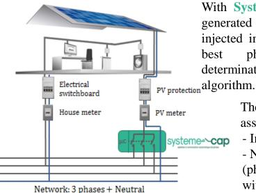
With Systeme CAP, power generated by solar panels is injected in real time on the previously phase determinated by the
