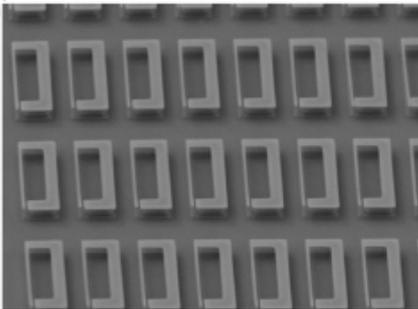
Dense array of identical THz resonators
