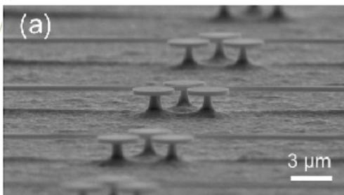
Sets of 3 GaAs resonators and their optical-coupling waveguides.
