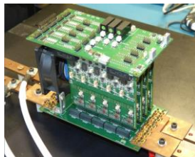
Multiphase 25-cell GaN interleaved converter (Vin=12-48V Vout=1-12V, 5x75A, Fsw =0.5-3MHz)
