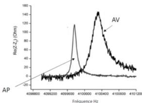
Frequency shift of the resonator while solid particles impact the surface
