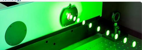
An autofocus system for femto/pico second pulsed lasers based on the coherence between incident and reflected light from the sample.
