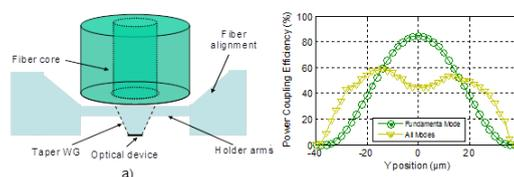
Coupling efficiency, with optical fiber fundamental mode (green) or with a uniform energy distribution representing worst case (yellow) © Jean-Luc Polleux
